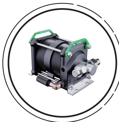
The HFLG series air driven liquid pumps developed by HiFluid use compressed air as the driving source to pressurize liquid media to the required pressure levels. Designed for a wide range of liquids—including oil, water, and other special fluids—the pumps can achieve maximum output pressures of up to 600Mpa.
