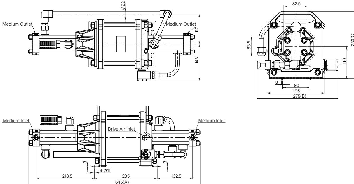
The single-drive two-stage gas booster can boost lower-pressure gases, comparing to single-drive double-acting models under the same pressure ratio. With two different pressure stages for a secondary boost, it could effectively boost the inlet low-pressure medium gas to a higher pressure. HiFluid offers six different pressure ratios to meet applications where the initial pressure of the medium gas is low, but it needs to be boosted to a higher pressure.
