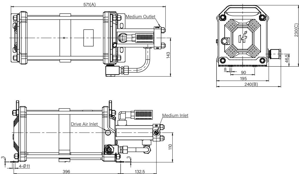
The double-drive double-acting gas booster not only pump larger volume of a Single Acting Booster per cycle, but also require less air drive since the inlet gas pressure is assisting the air drive in each direction. HiFluid offers four different pressure ratios for applications requiring higher flow rates.
