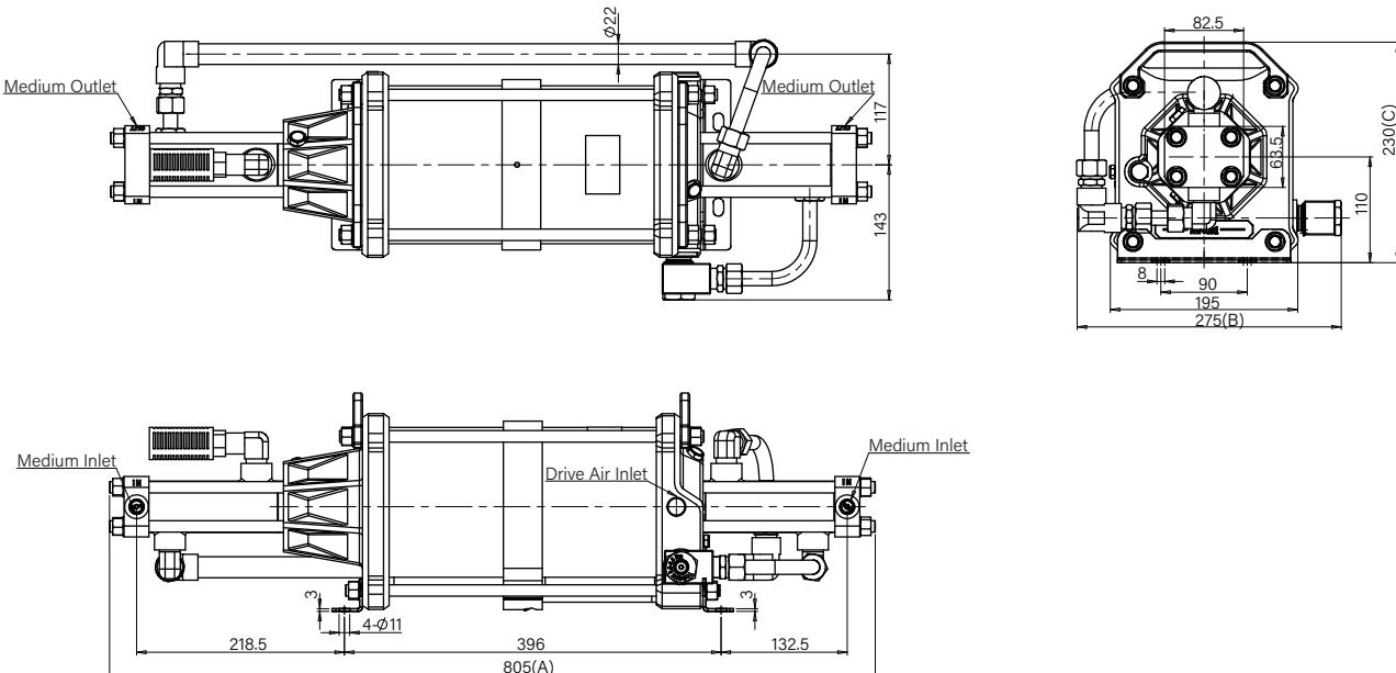
The double-drive two-stage gas booster can boost lower-pressure gases, comparing to double-drive double-acting models under the same pressure ratio. With two different pressure stages for a secondary boost, it could effectively boost the inlet low-pressure medium gas to a higher pressure. HiFluid offers six different pressure ratios to meet applications where the initial pressure of the medium gas is low, but it needs to be boosted to a higher pressure.
