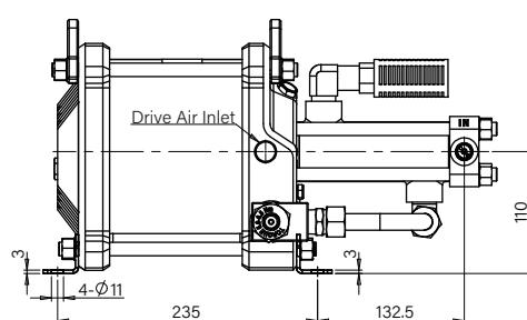
The single-drive double-acting gas booster not only pump larger volume of a Single Acting Booster per cycle, but also require less air drive since the inlet gas pressure is assisting the air drive in each direction. HiFluid offers six different pressure ratios for applications where pressure requirements are low but flow requirements are higher.
