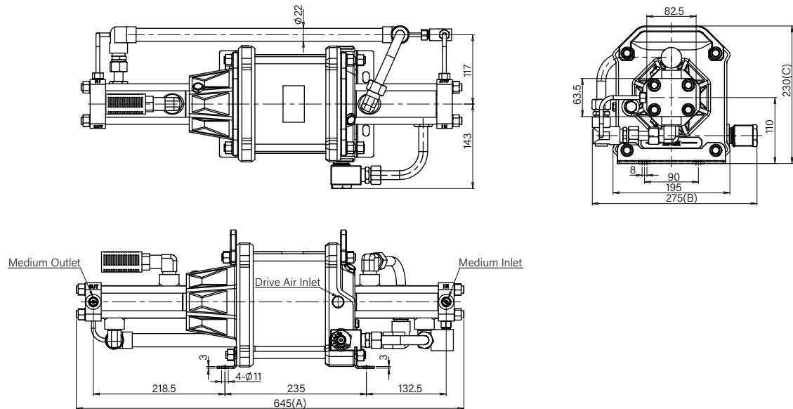
The double-drive single-acting gas booster has a larger flow rate compared to single-drive single-acting models under the same pressure ratio, but also consumes more compressed air. HiFluid offers four different pressure ratios for applications where the medium gas pressure requirement is relatively high.
