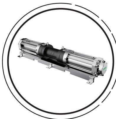
The HiFluid HFHG1 Series hydraulically driven gas boosters use low-pressure hydraulic oil as the driving source to boost process gases to the required pressure. The standard design supports a maximum working pressure of 17,000 psi, with special designs available for higher pressure requirements. These boosters are highly efficient for ultra-high-pressure and large-flow gas applications.
